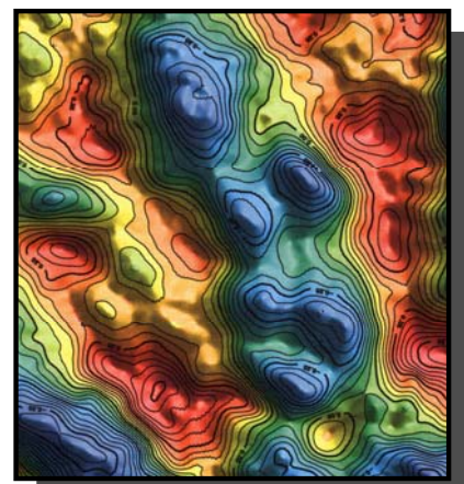
Typical Bouguer residual anomaly from a modern 3D gravity survey (contour interval 0.05mGal; horizontal dimension is 15 miles).
