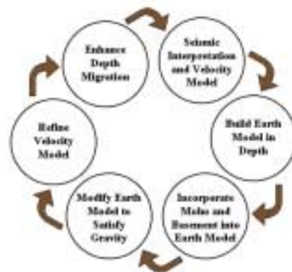
The process used generated a velocity model constrained by the combination of seismic and potential fields data in a single integrated earth model.
